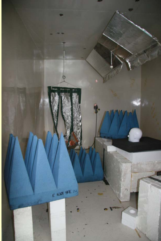
Reverberation chamber with absorbing material and phantom head
